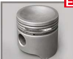
ROTURA DE LAS LANDAS / BREAKAGE OF THE RING LANDS BY MECHANICAL OVERLOAD
